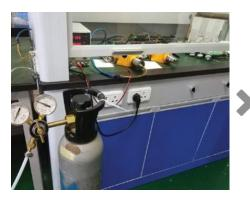
Factory Calibration The sensors are bump tested at Oizom factory to check their proper functioning for each parameter.
